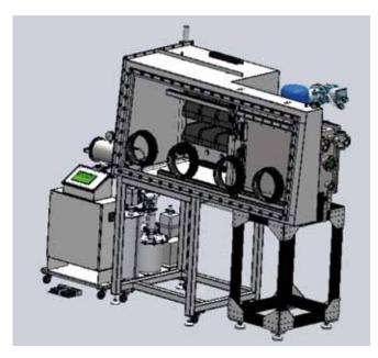
Figure 3: LC tech glovebox with our in-house integrated vacuum chamber designed to further develop the project.
